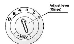
The rinse aid dispenser has six or four settings. Always start with the dispenser set on "4". If spots and poor drying are problems, increase the amount of rinse aid dispensed by removing the dispenser lid and rotating the dial to "5". If the dishes still are not drying properly or are spotted, adjust the dial to the next higher number until your dishes are spot-free. The recommended setting is "4". (Factory value is "4".)
